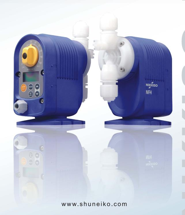
The series NFH is a solenoid driven metering with the concept of the user-friendly design. Our technology makes the pump with reliable feeding performance. The feeding capacity can be adjusted via stroke length and stroke frequency to obtain a satisfied turndown ratio.
